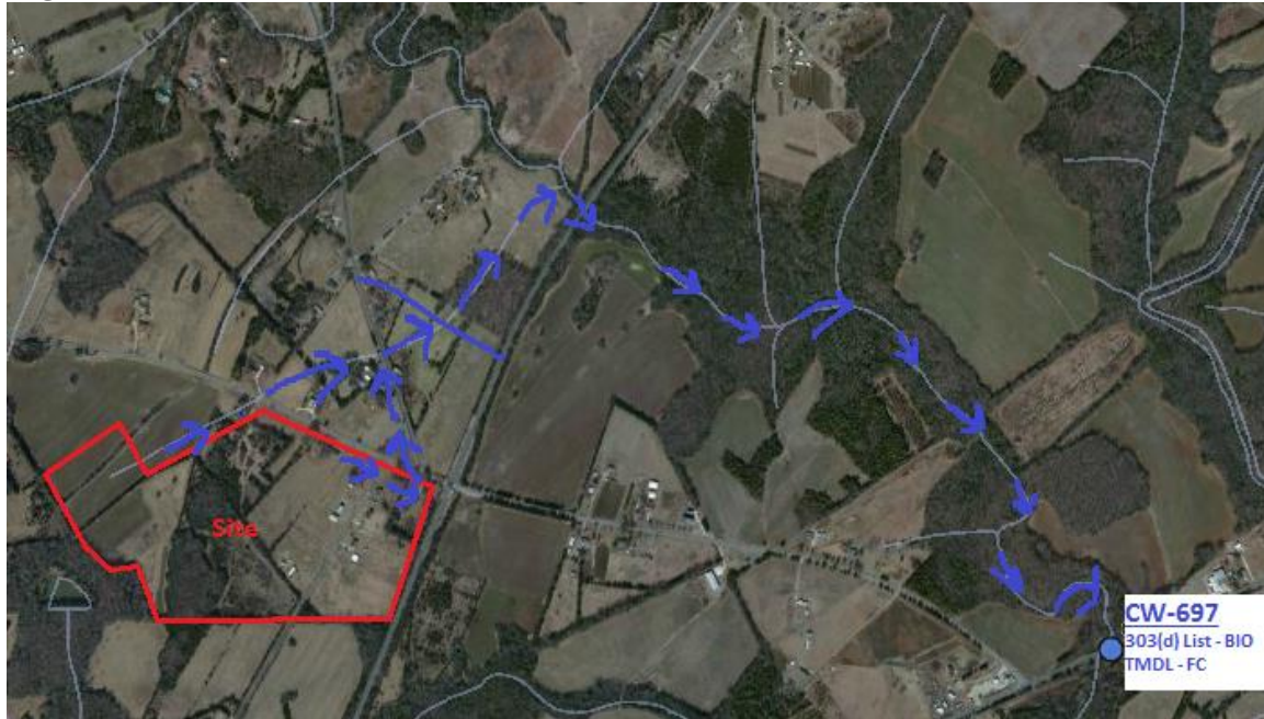
Figure 2.2: Stormwater Runoff Route
