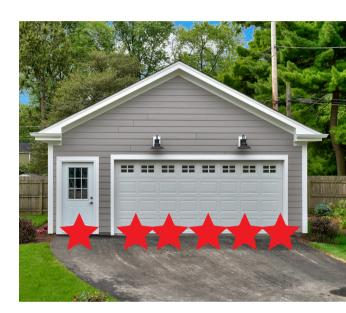
Sandbags should be used at any entryway to your home, including doors and garages (as indicated by the red stars). Bags should be placed parallel to the direction of the water flow.
